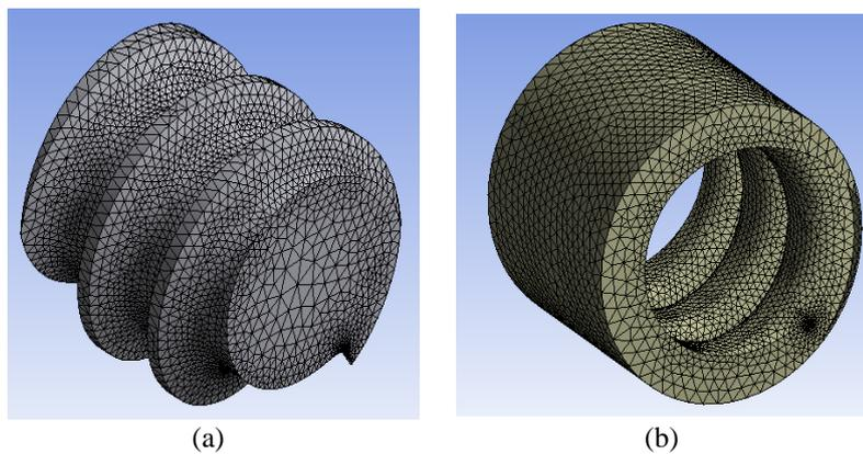
**Figure 3** ANSYS meshing (a) screw, (b) barrel.
