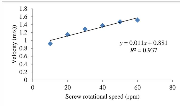
**Figure 7** Simulation of relationship between screw rotational speed and velocity.
