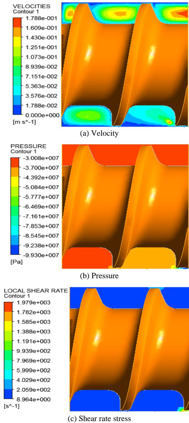
**Figure 4** Contour map of model screw.
